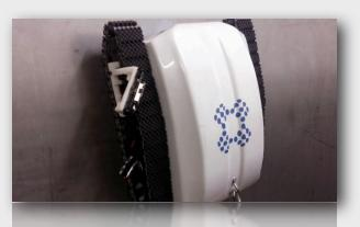
is created by Christchurch robotics company Invert Robotics and was originally designed for use in the dairy industry to detect damage inside milk tanks. The remote controlled robots have the ability to climb walls and stream high resolution footage in real time.
